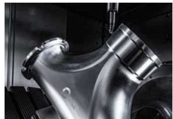
top Complex shapes accurately machined: A fuel connector after the roughing process on a C 32 U dynamic.
